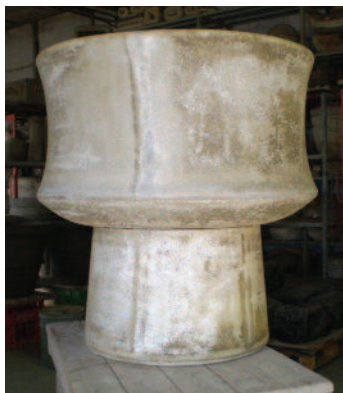
Jackpot (24" diameter at the top) just before being fired at the Italian factory. It will turn rosy pink after firing.
